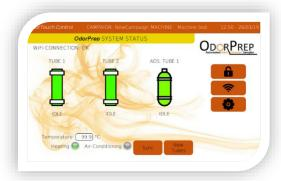
Sampling can be performed manually too. OdorPrep® system may be activated in the field by accessing the on-board computer, equipped with the dedicated management software.
